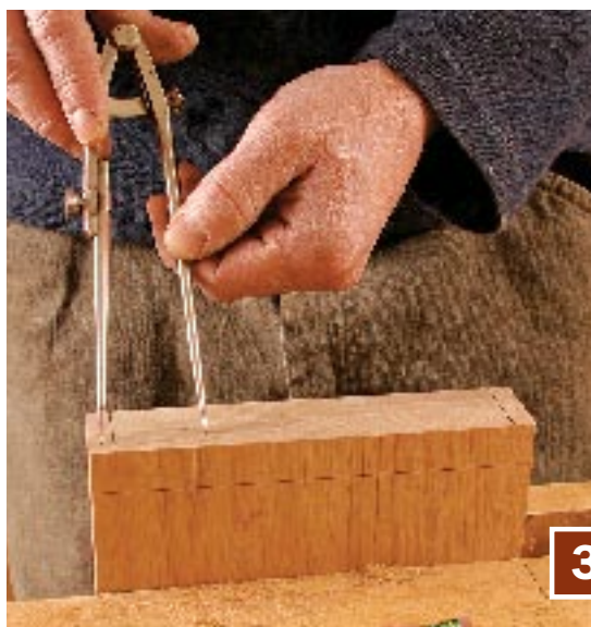
1 Mark the pin width. Stack both tail boards in the vise. After laying out half-pins, mark the pin width on one end.
