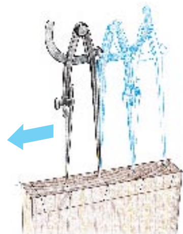
3 Mark the left edges of the tails. Place one point of the dividers on the right half-pin line and walk the dividers across the end grain.
