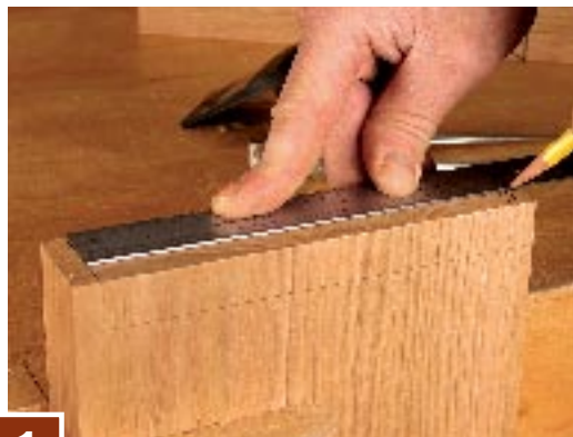
1 Mark the pin width. Stack both tail boards in the vise. After laying out half-pins, mark the pin width on one end.
