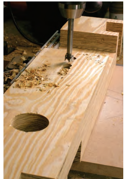
Holes to guide you. The through-mortise in the leg allows the parallel guide to pass freely in and out. You don't need to square the ends of this mortise. Leave them round. The parallel guide is narrow enough to pass through.
