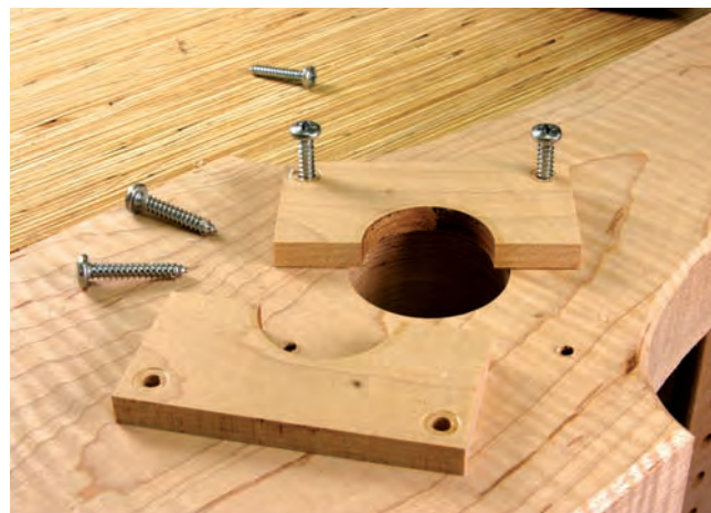
Garter, disassembled. To assemble the leg vise, drop the vise screw through the hole in the chop and fit the garter in its groove. Screw the garter pieces down and you're ready to bust some walnuts with your vise.
