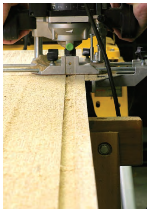
Wear a dust mask. When you rout LVL, the misery begins. The stuff kicks up a lot of stinky, fine, super-nasty dust. Wear a good dust mask, even if you normally throw caution to the wind.
