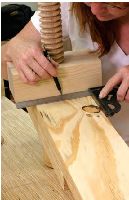
Snug, square and traced. Put the vise screw through the 2" hole and snug up the vise block on the backside of your leg. Square up the block then trace its outline on the leg.
